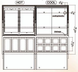
2 1/2" HOLE REQUIRED FOR COOLING AND DRAINAGE LINES
